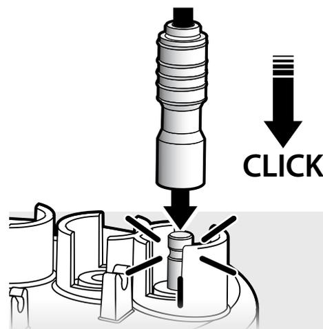
**Fast maintenance: quick connectors for the power supply ensure easy, fast and safe cylinder replacement.**
